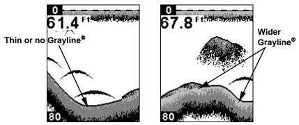
At left, little Grayline indicates a soft bottom, probably sand or mud. At right, the wider Grayline indicates a harder, rocky bottom.
